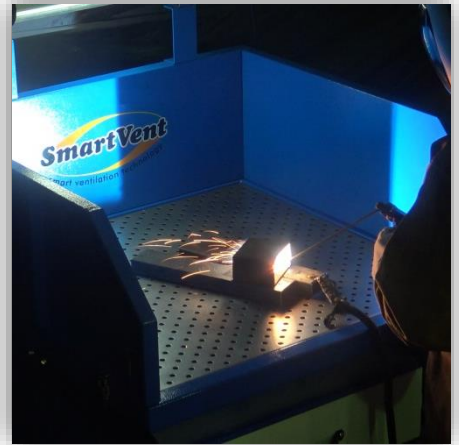
Welding Fume Extraction
