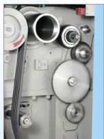
▲ Multiple threading system for cutting worm.
